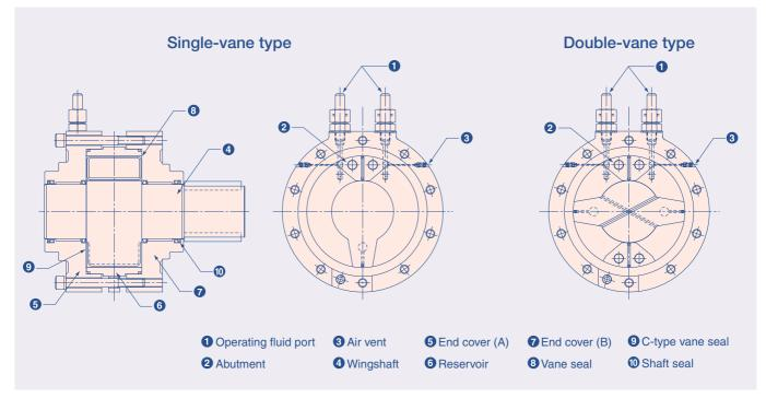
Note: The number of keys of the wingshaft is one in the single-vane type, and two in the double-vane type.
